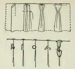
The making of a French plait is shown in the drawing above, and below are different ways of fastening curtains to rods.
